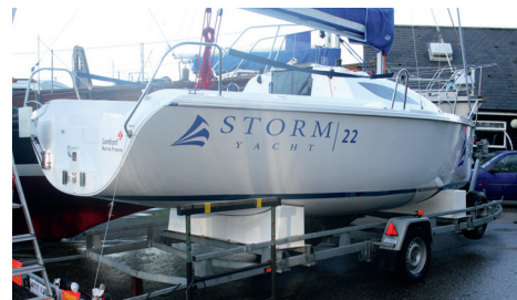
The 22 sits comfortably on a two-wheeled braked trailer and can be towed with a medium-sized 1800cc or two-litre family saloon.
